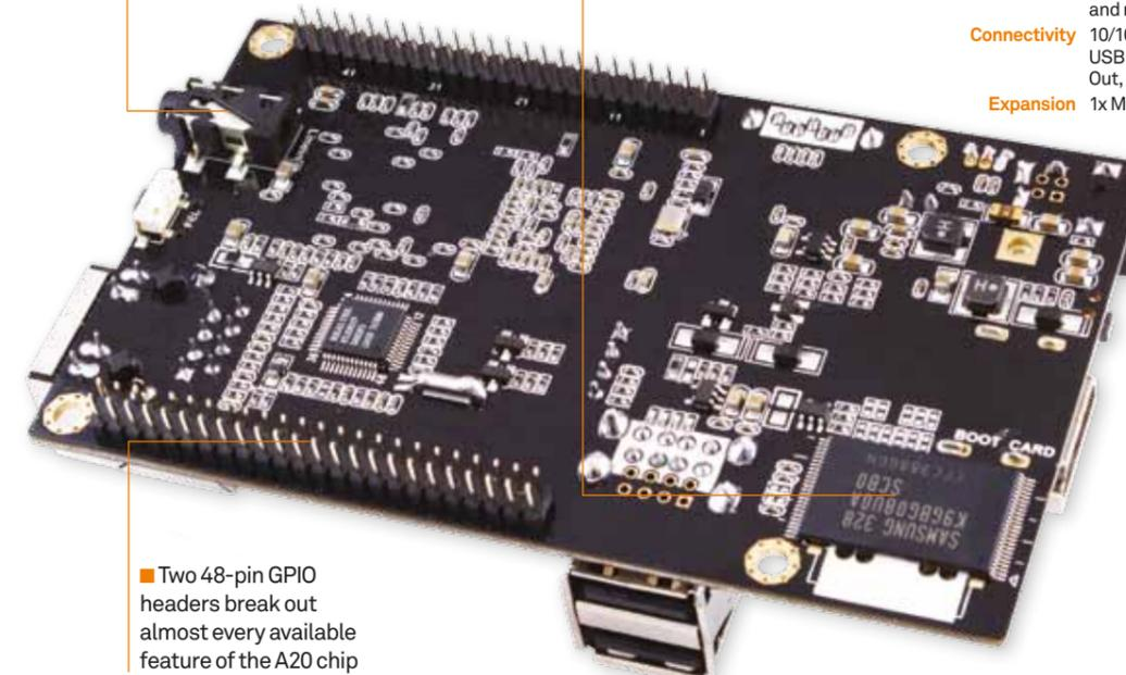
Two 48-pin GPIO headers break out almost every available feature of the A20 chip
