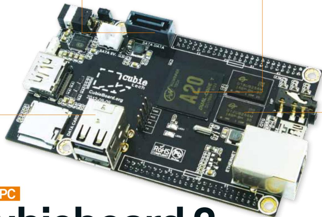
As well as analogue audio output, the Cubieboard 2 includes line-in, and SPDIF digital audio via the GPIO header
